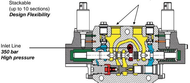
Priority Flow Sharing **Prevents loss of controllability Elimination of bleed off Machine efficiency**
