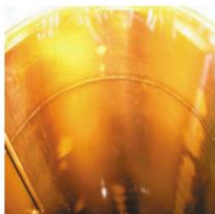
Journal bearing failure
