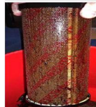
Plugging of filters
